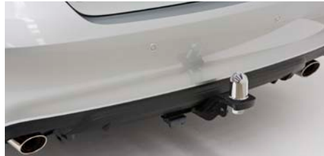
Towbar. The fixed tongue towbar and accessories allow you to tow a maximum braked load of 1200kg and unbraked load of 500kg with your Camry.
