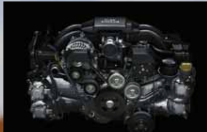
The 86's 2.0L front boxer engine has D-4S direct injection to provide you with power when you need it. The engine achieves a 147kW @ 7,000 rpm and has 205Nm of torque @ 6400-6600 rpm. At 5000 revs the car's attitude changes and it's on!
